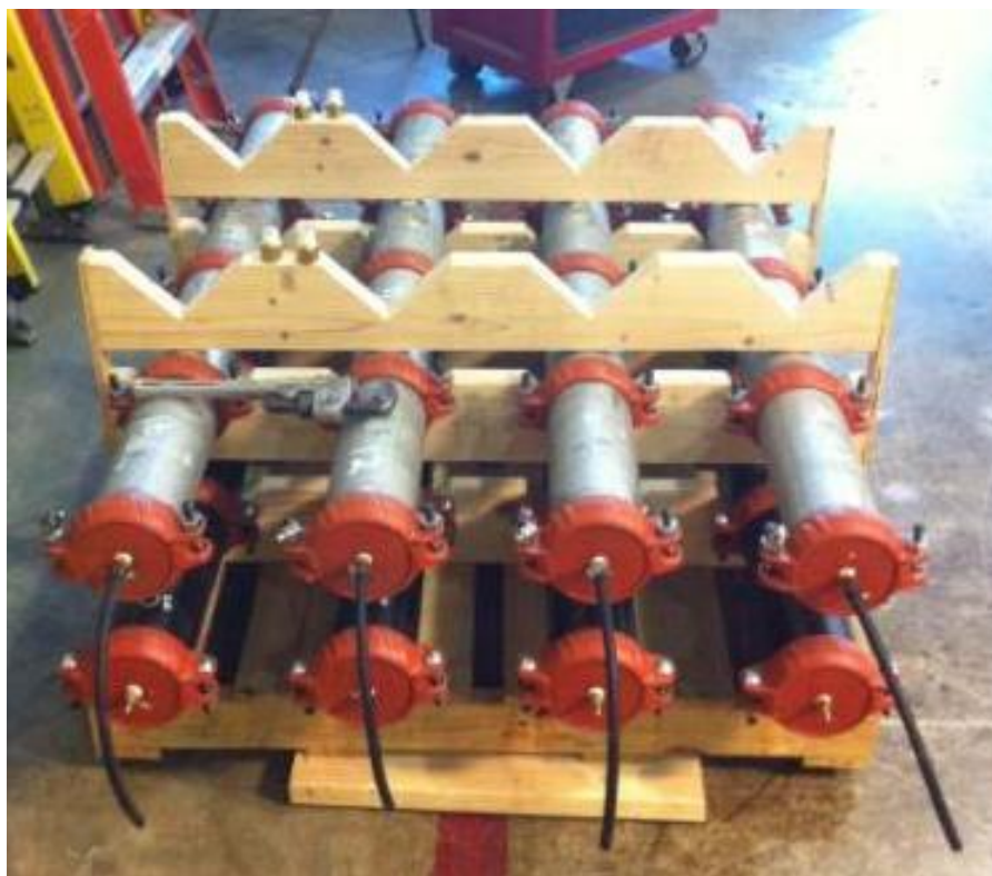
Corrosion Comparison Tests
